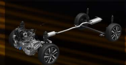
MacPherson Strut & H-Shape Torsion Beam Suspension
